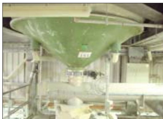
Stainless steel bulk silo(T42), cap.: 90 m3, on weighing indicators
