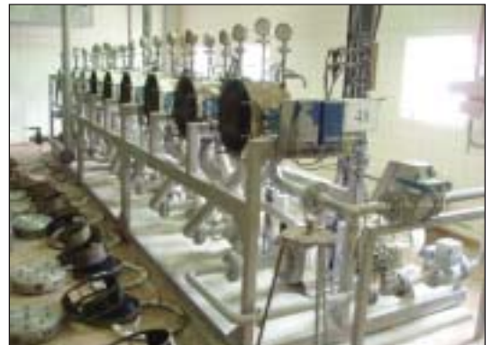
Dorr Olivier tenfold gluten cyclone plant with Salsa Delta centrifugal pumps Dorr Olivier 10-voudige gluten cycloneninstallatie v.v. Salsa Delta centrifugaalpomp
