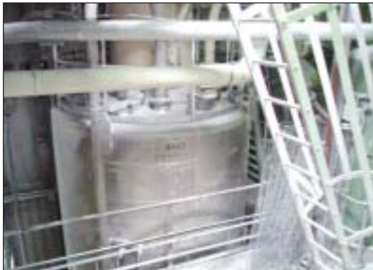
Ss bulk silo (50-T-46), full cap.: 60 m 3 with free fall valve (50x83)
