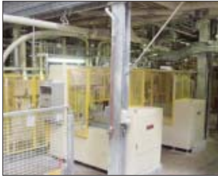
Bran & Luebbe Concetti valve bag filling plant, type: Minipond 25, serial nr.: 5089, cap.: ca. 25 ton/h.
