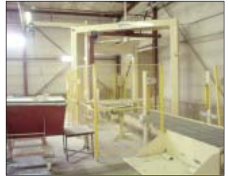
Matco pallet foil wrapping machine, type: ALS-TSD, max. load: 1.500 kg.
