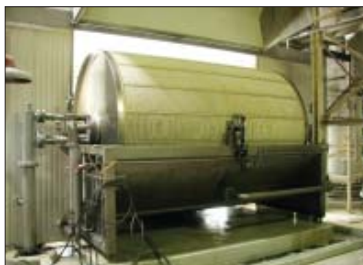
Hovex stainless steel vacuum cloth drum filter, type: F2400-320, with wet mill, cap.: 30 kW.
