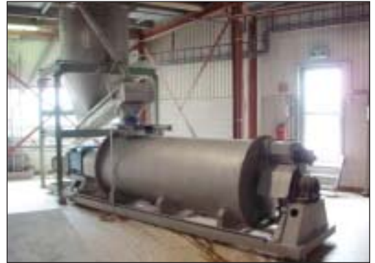
Stainless steel buffer hopper-/wheat flour kneading machine, cap.: 2 m 3 , Rvs bufferkaar-/tarwebloemkneedmachine, cap. inhoud: 2 m 3
