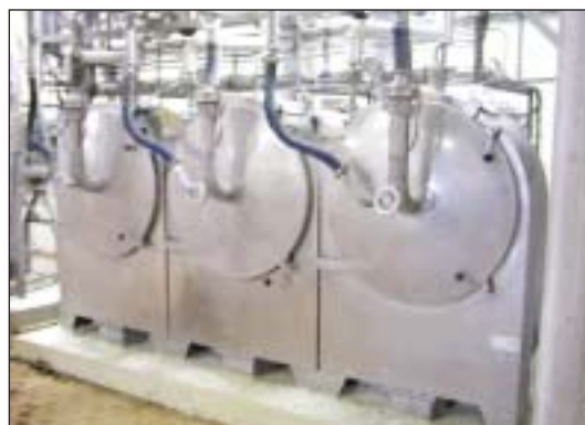
Lot with 3 G-Larssons stainless steel centri sieves, ymf: 2001, machine type: GL 850
