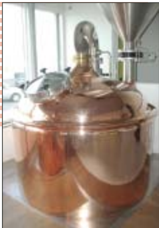
brouwketel brewing boiler Braukessel
