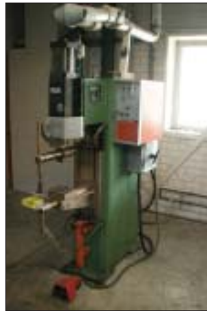
Harding puntlas-machine/spot welder, model: WP 125 RL, cap.: 125 kVa
