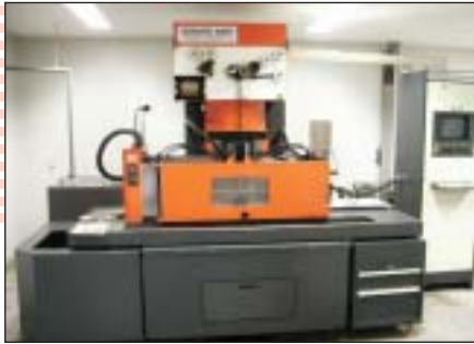
Charmilles draadvonkerodeermachine/wire erosion machine, model: Robofil 6000
