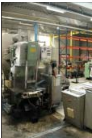
perslijn/press line: Arku afwikkelhaspel/de-coiler, Arku richtwals/straightening roller, Paul Müller excenterpers/ex-centre press, cap.: 80 t.
