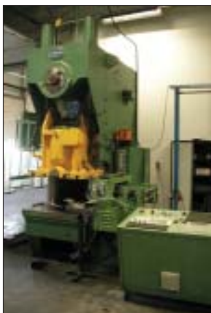
perslijn/press line: Cordt afwikkelhaspel/de-coiler, Hoffmann richtwals/straightening roller, IWK pers/press, cap.: 160 t., met/with feeder
