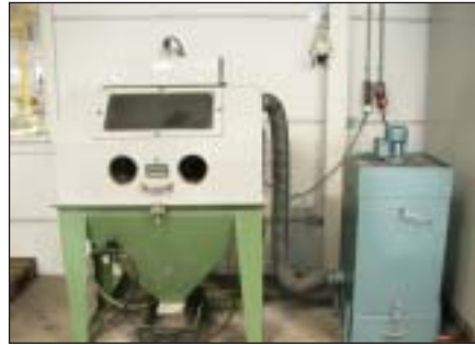
Econoline straalcabinet/blast cabinet, model: RA 42x24
