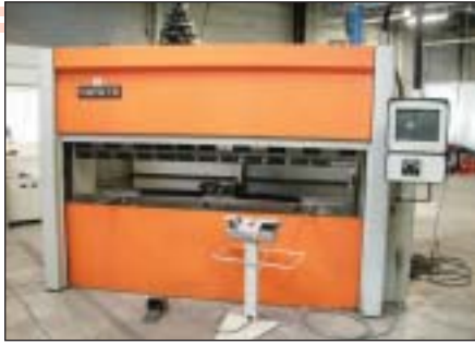
Safan servo hydr. CNC kantbank/servo hydr. brake press, model: PLCS 110-31200TS2, cap.: 110 t./3.100 mm.
