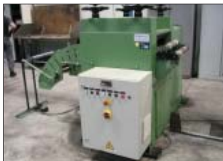
perslijn/press line: Cordt afwikkelhaspel/de-coiler, Hoffmann richtwals/straightening roller, IWK pers/press, cap.: 160 t., met/with feeder
