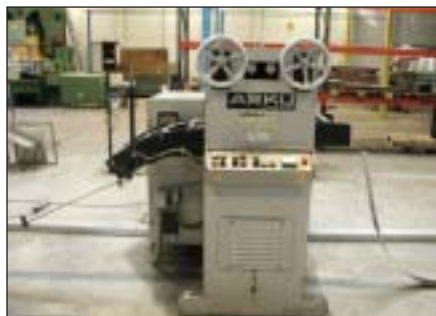
perslijn/press line: Arku afwikkelhaspel/de-coiler, Arku richtwals/straightening roller, Paul Müller excenterpers/ex-centre press, cap.: 80 t.
