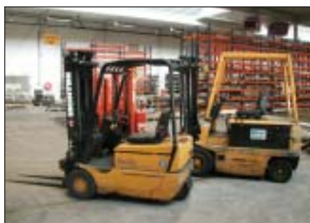
Montini vorkheftrucks/fork lift trucks, cap.: 1.500 and 2.500 kg.
