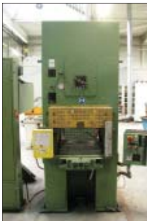
Paul Müller kolompers/column press, model: HSP 25, cap.: 25 t.
