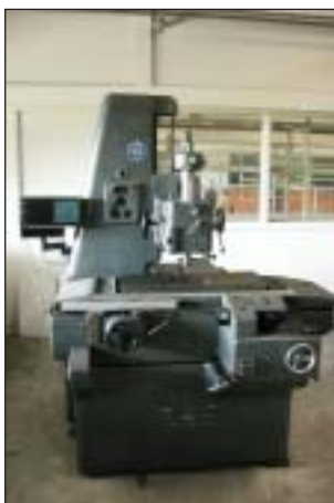
S.I.P. coördinaten boormachine/co-ordinate drill, model: MP-2P
