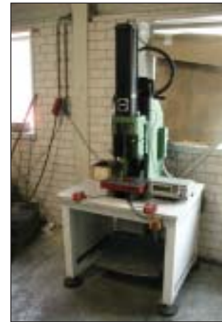
Haeger klinkpersen/riveting press, model: HP6C
