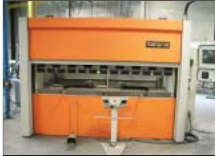
Safan servo hydr. CNC kantbank/servo hydr. brake press, model: SMK 50-2550TS1, cap.: 50 t./2.550 mm.,
