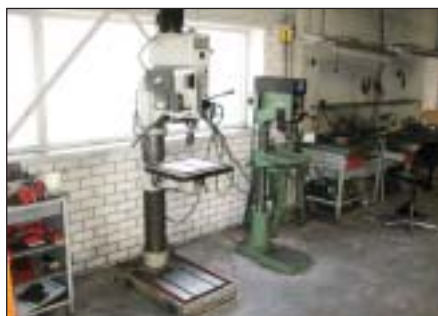
kolomboormachine/column drilling machines
