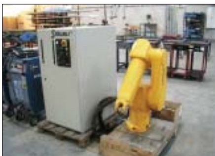
Staubli lasrobotarm/welding robot, model: RX 90
