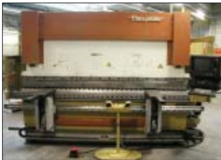
Beijeler kantbank/brake press, met/with bombeerinrichting/crowning compensator
