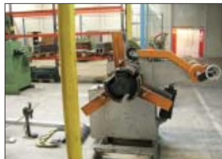
perslijn/press line: Arku afwikkelhaspel/de-coiler, Arku richtwals/straightening roller, Paul Müller excenterpers/ex-centre press, cap.: 80 t.
