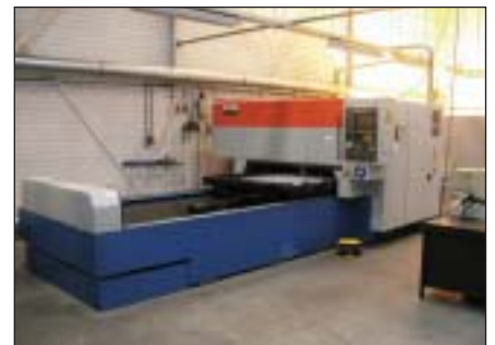
Mazak CNC lasersnijmachine/CNC laser cutting machine, model: Super Turbo X510 Hi Pro, cap.: 2 kW.
