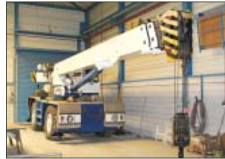
Coles Mobile Crane model: Husky 635, cap.: 30,5 tons
