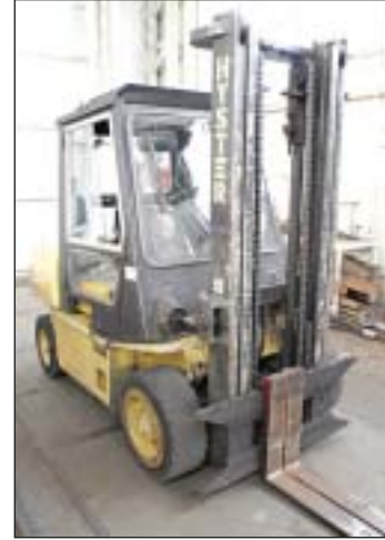
Hyster Fork-Lift Truck, cap.: 4 ton/3700mm
