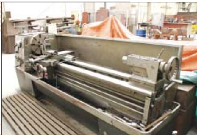
Colchester Lathe model: Mascot 1600
