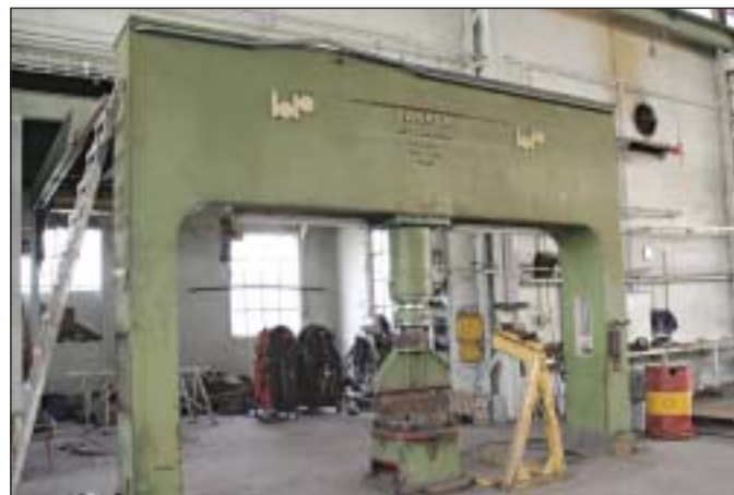
Bakker Hydraulic Press, cap.: 200 tons
