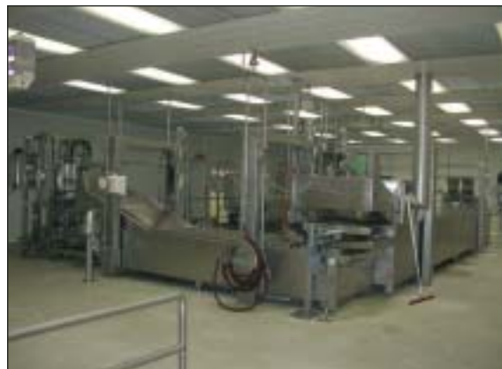
rvs kookbad en rvs koelbad/ stainless steel cooking tub and stainless steel cooling tub
