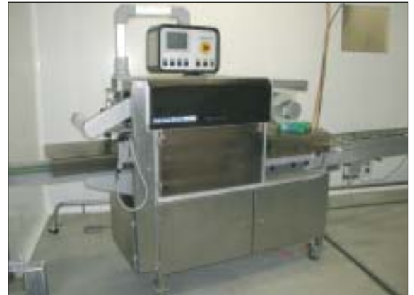
Sealpac rvs sealmachine 610/ Sealpac stainless steel sealing machine 610
