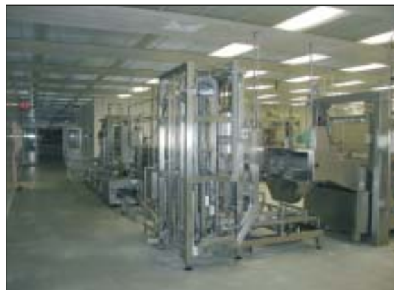
rvs kratten transport en was installatie/ stainless steel crates transportation and washing installation
