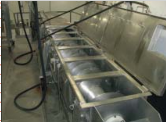
rvs schroef pasteur / stainless steel screw pasteurizer
