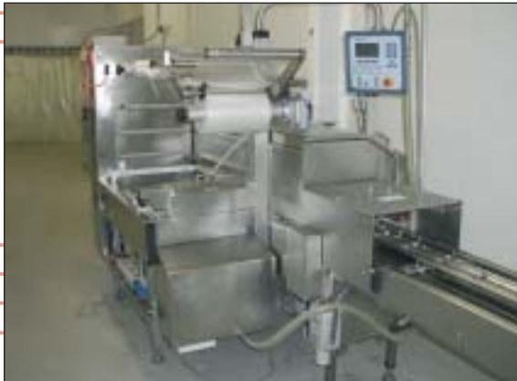
Multivac rvs vacuümverpakkingsmachine T 400/ Multivac stainless steel vacuum packaging machine T 400
